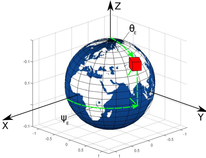
**Figure 2:** Earth-Centered Inertial Frame and Spherical Coordinate Frame
