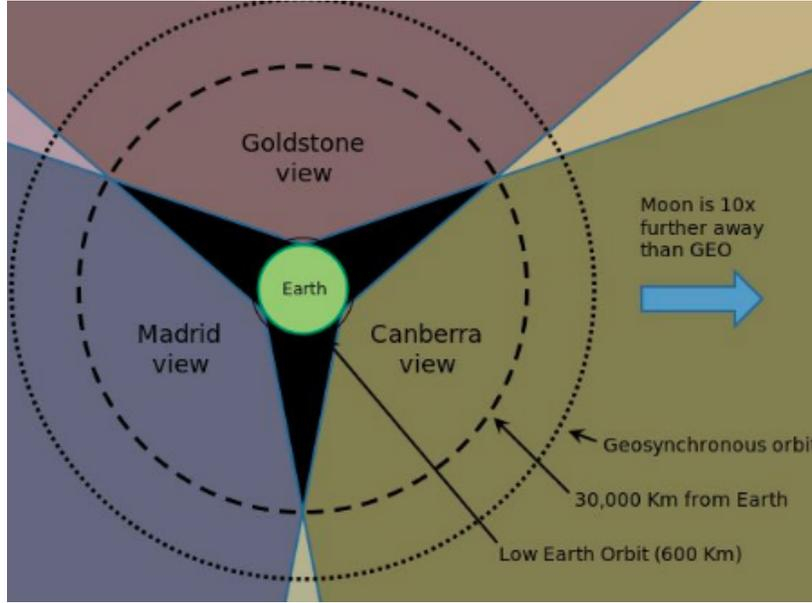
Figure 11: Deep Space Network Satellite Coverage [34]
