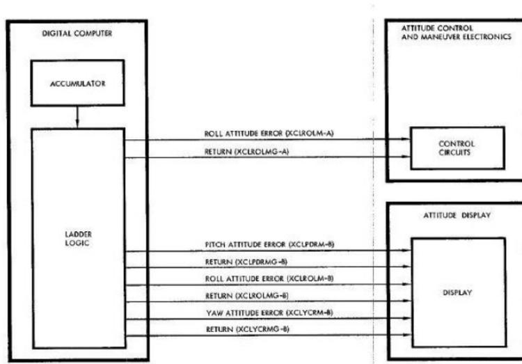
**Figure 13:** ACME Interface Diagram from the Gemini Spacecraft[43]
