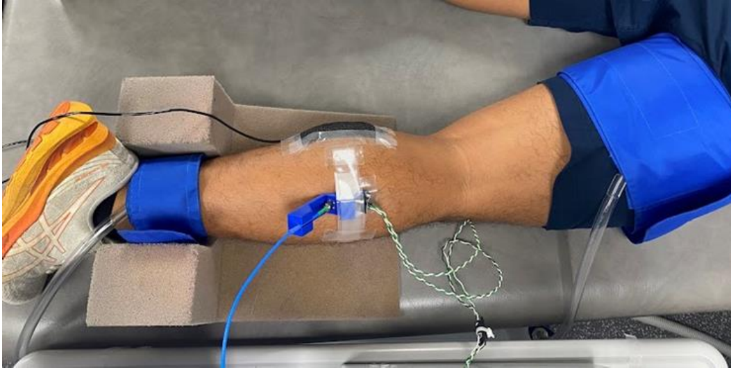
Figure 3. Experimental setup. The REFLO and NIRS devices are secured to opposite sides of the lateral calf with clear medical tape. The REFLO transducer is connected to the Arduino microcontroller and REFLO transmitter (out of frame). Cuffs are secured at the ankle and upper thigh for the vascular occlusion protocol.
