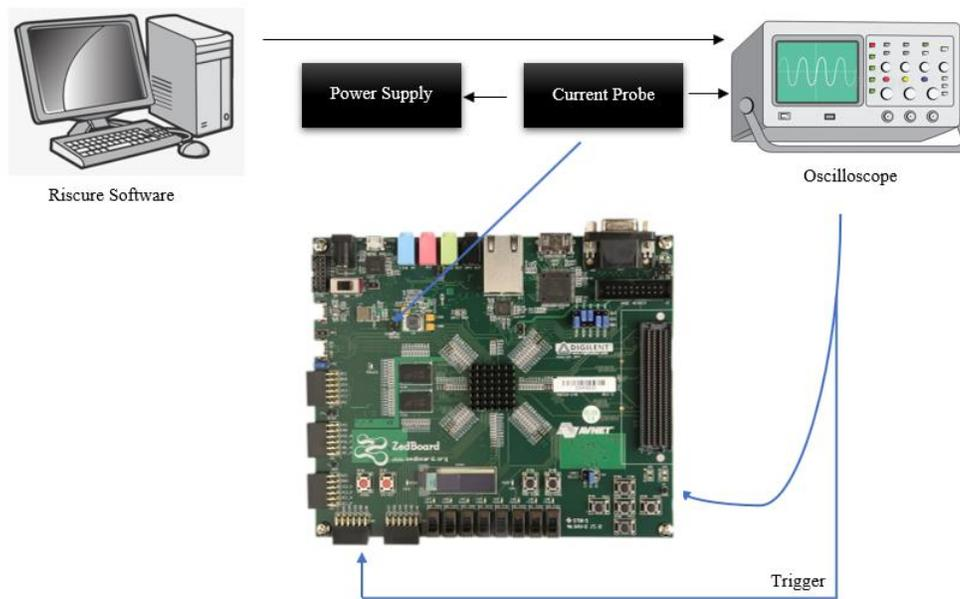
Figure 3.4 System Under Test (SUT).
