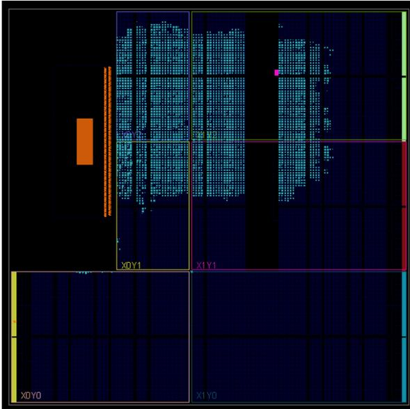
Figure 4.6 Device View: Variant DES\_20 without Optimization.
